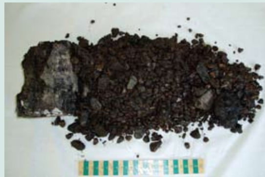
Figure 4.1 Core showing binder stripping in A3052
