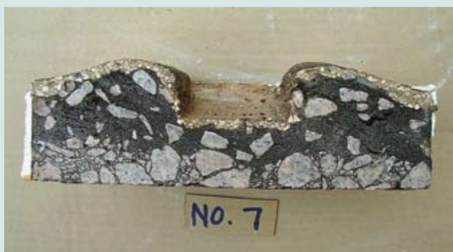
Figure 3.1 HRA deforming in wheel-tracking test
